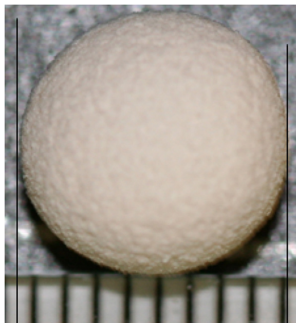
Fig. 2. Typical example of a brittle test particle (diameter of test particle 8.6 mm).
